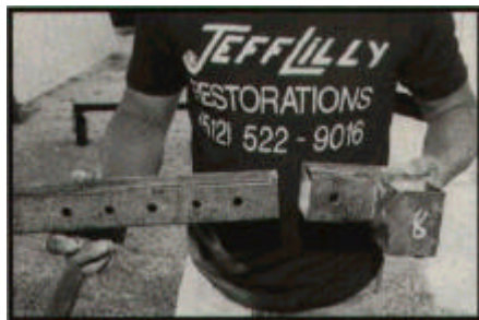
21 Place the adjustment sliders #7 and #8 onto the arms #2.
